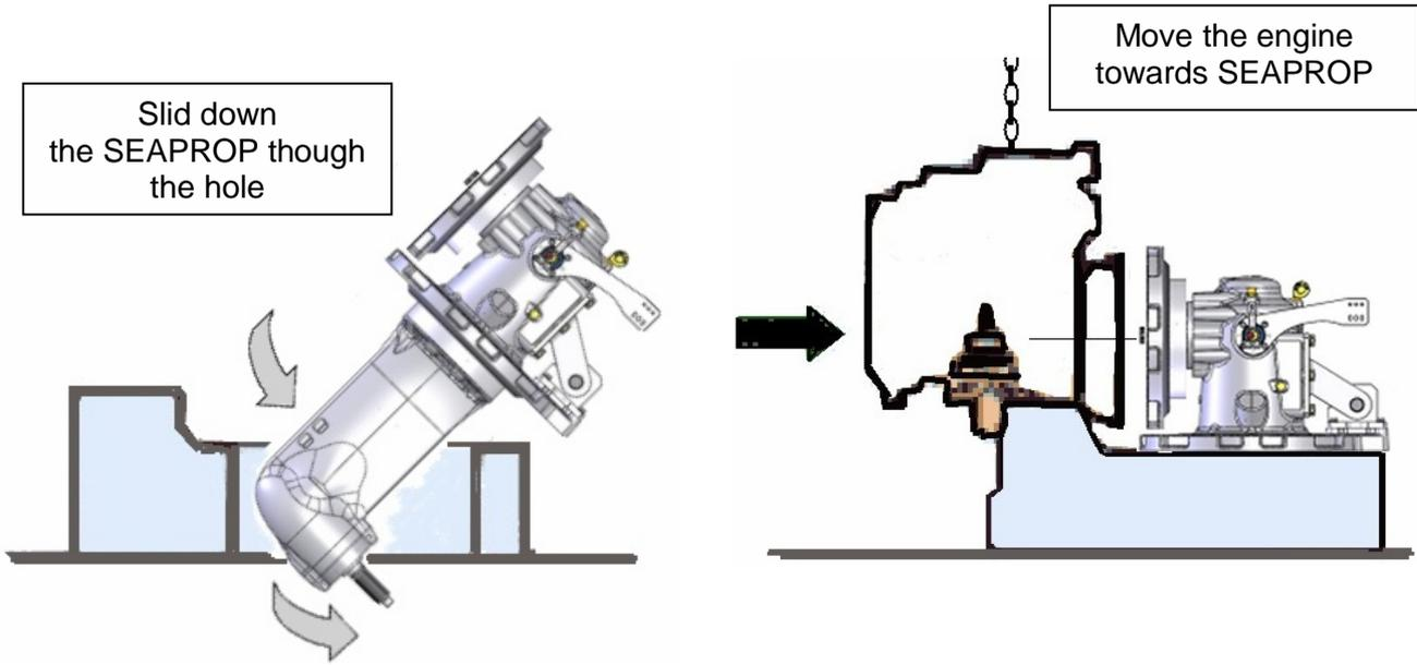
Place the thru-hull flange onto the engine bed so that it matches with the studs or the bolt bores. Crew nuts or bolts but do not tighten. The resilient mounting racket can be fitted, but do not tighten the clamp yet.
