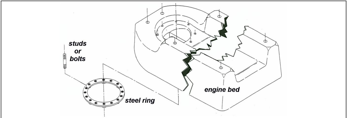
Once the hull is even with the floor, identify the location of the engine bedding in the hull and proceed with markings:
