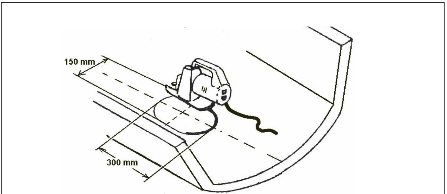
The Engine bed is glassed to the hull both around the outside of the bed, and around the hole cut in the hull for the drive leg, as shown in this diagram. Photo's of the process follow.
