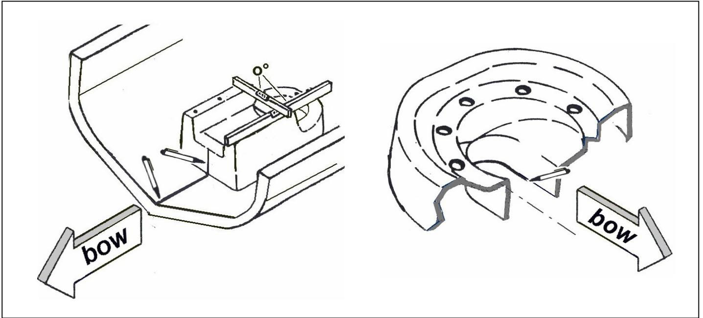
Once marked, remove the engine bed and cut
